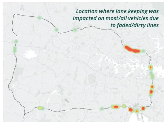
Location where lane keeping was impacted on most/all vehicles due to faded/dirty lines
